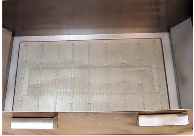
Support grid properly placed in filter pan.
